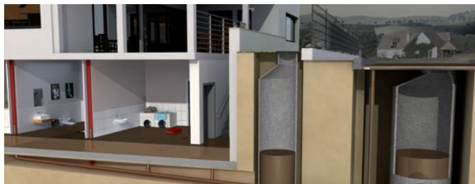
Without backpressure prevention (see page 75 for animations in the PumpSizer app)
