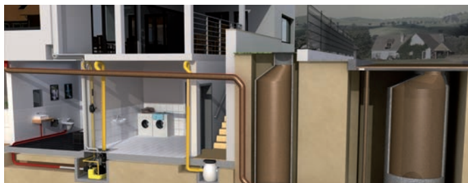
With backpressure prevention (lifting station)
