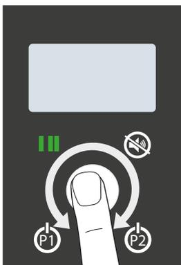
The individual menu options / parameters are set using the rotary switch.
