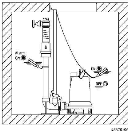
**Installation:** Fix the coupling base firmly to the floor of the collection chamber using wall plugs and then mount the guide rail. Next, install the pressure pipe including the necessary fittings, such as the non-return valve and shut-off valves.
