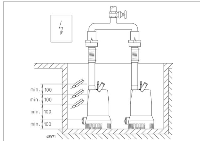
**NOTICE!** The floats of the level control and alarm system are installed so that they are freely movable but not under the inlet. Please observe the minimum distances. The controls must only be installed in a dry and well ventilated room!
